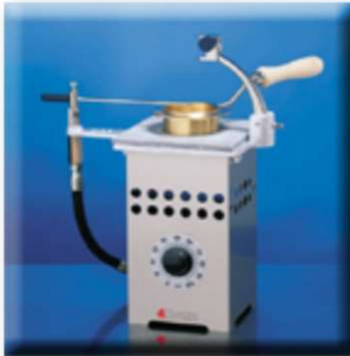
Cleveland open cup for flash and fire points of petroleum products, except fuel oils and those having an open cup flash below 79°C (175°F).
