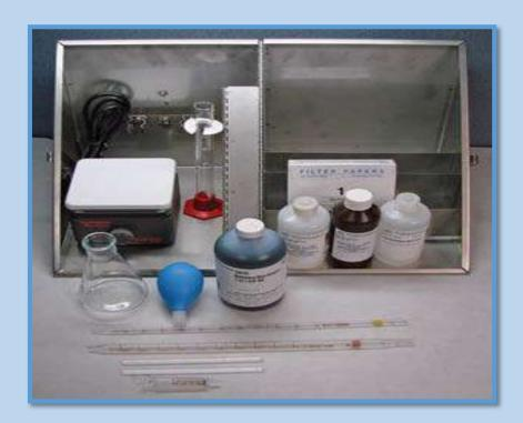
**Purpose**: The methylene blue capacity of a drilling fluid is an indication of the amount of reactive clays (bentonite or drilled solids) present as determined by the methylene blue test (MBT)
