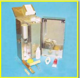
Purpose: Determination of water, oil &solid content in drilling mud
